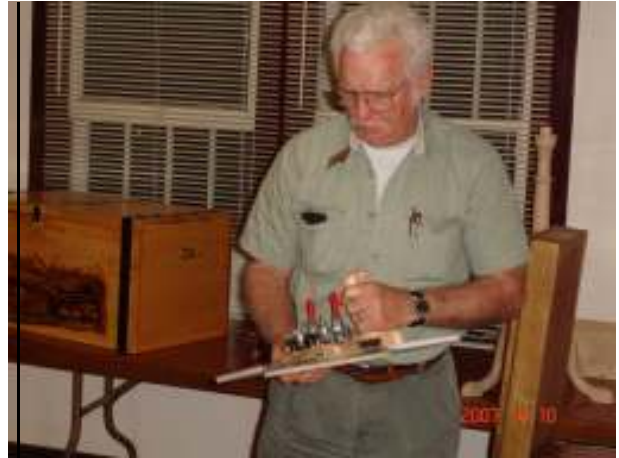
Art Peasall shows us a sled he made to hold small parts safely. He uses it on the router table and his table saw.
